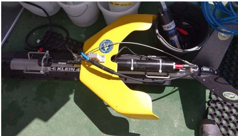
Fig. 5.1.2 Sidescan system with mounted USBL positioning system
