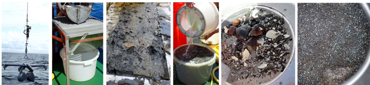
Fig. 5.10.1 Photos illustrating sampling procedure. The two right-most photos show the fractions left on the 1.0 mm and 0.5 mm sieves.
