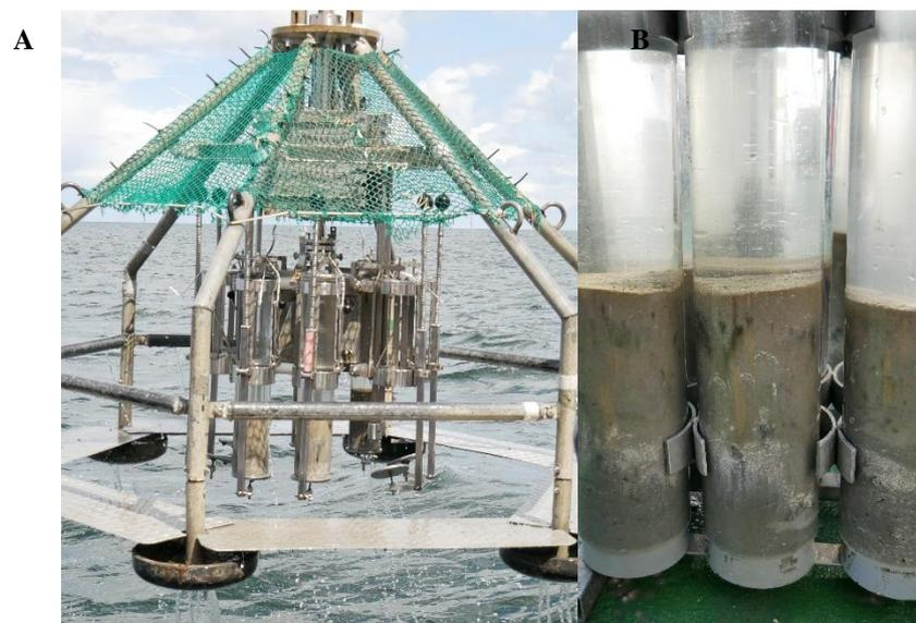
**Fig. 5.5.1** A Sample collection using multicorer equipped with 4 corers. B Detail of the corers at station EMB342\_13\_6.
