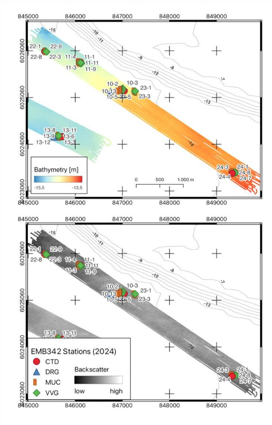
**Fig. 5.1.4** Bathymetric (upper) and backscatter (lower) map with hillshade of the MPA at Oder Bank area. No trawl marks are visible in the data.
