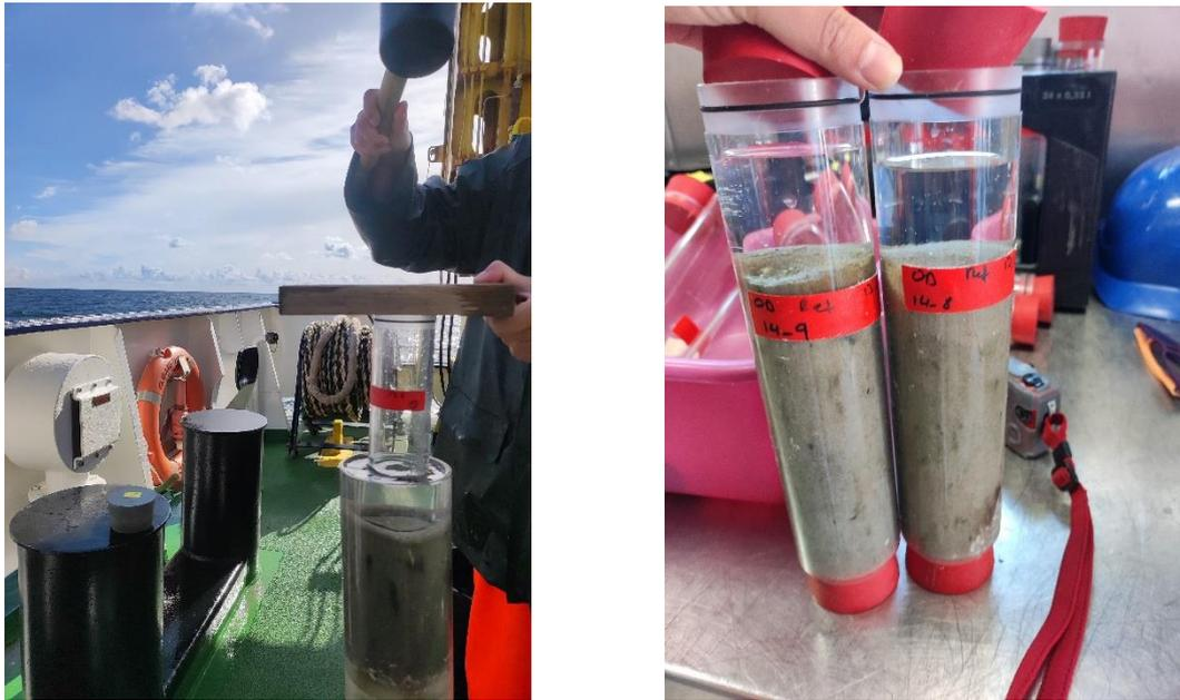
**Fig. 5.4.1** Sampling in Oderbank (5 cm Ø) from Multi corer cores 10 cm Ø
