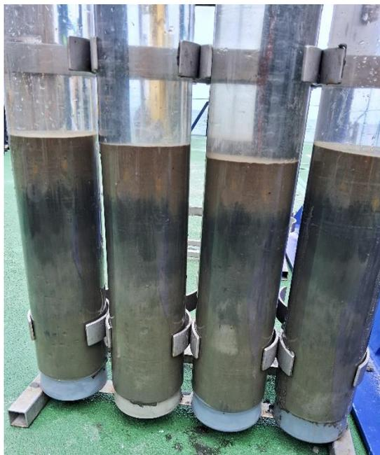
**Fig. 5.2.1.1** Parallel MUC cores collected from station 18-5 for benthic geochemical study; show black layered sediment below the surface.
