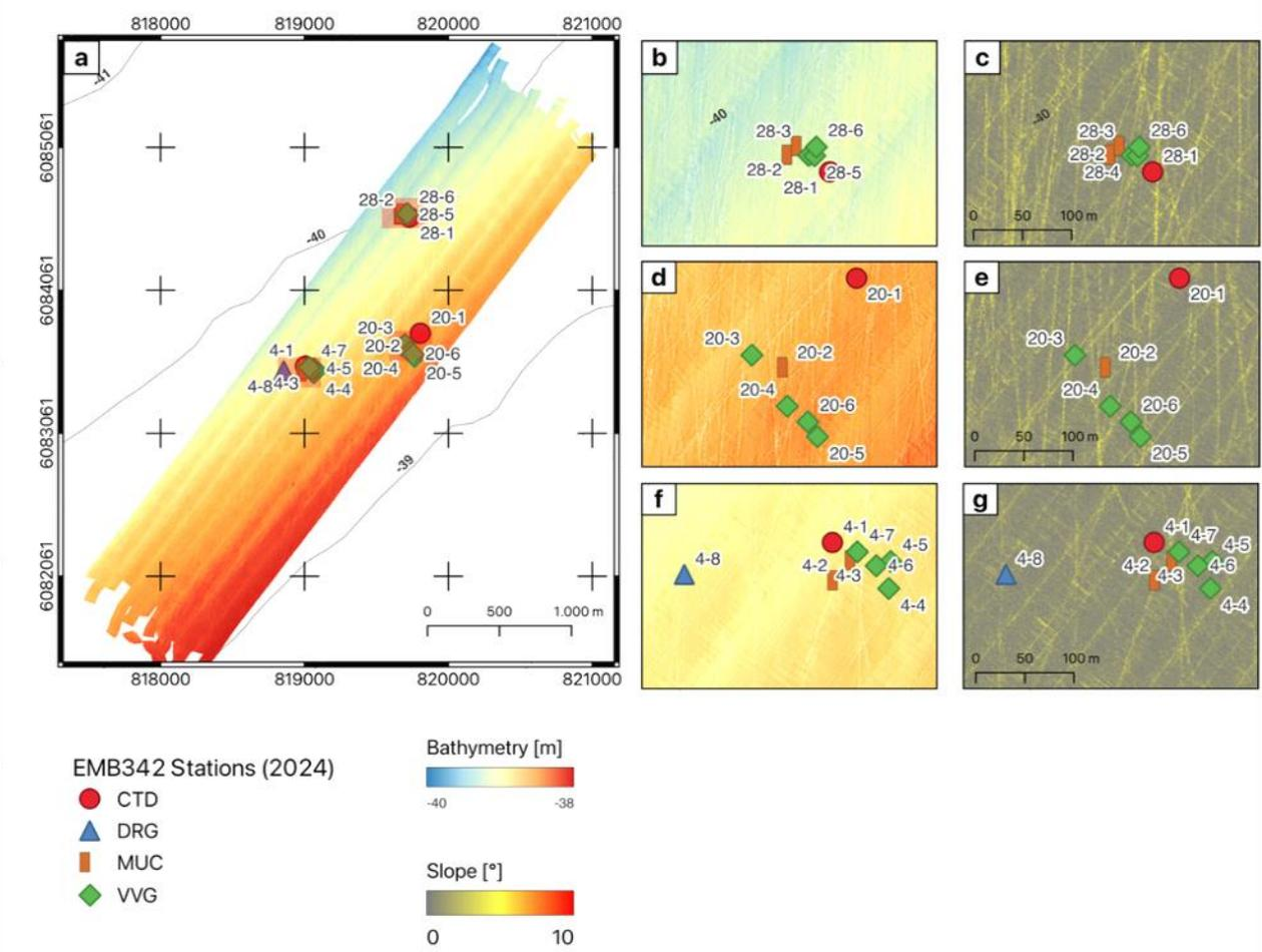
**Fig. 5.1.2** (a) Bathymetric map of the REF area at Rönne Bank area. The impact of trawl tracks on the seafloor surface is clearly visible in the bathymetry with hillshading (b, d, f) and slope data (c, e, g) at the respective stations.
