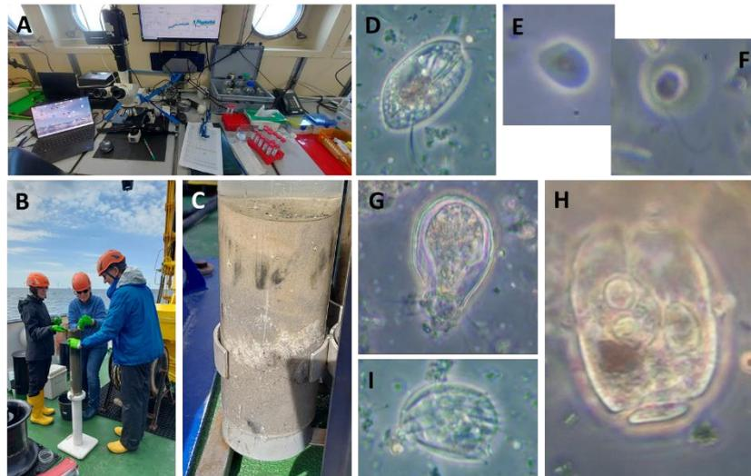
**Fig. 5.3.1** Live-counting of protists on board. A – Microscopic investigation by video-microscopy; B - Core slicing for subsequent live-counting, and cultivation of sediment samples; C – typical core from *Oderbank*; D – H different heterotrophic protozoan species observed during live-counting; D – colourless euglenid flagellate; E – goniomonads flagellate; F – *Metromonas* sp.; G – Testaceafilosea; H – heterotrophic dinoflagellate; I – *Aspidisca* ciliate.
