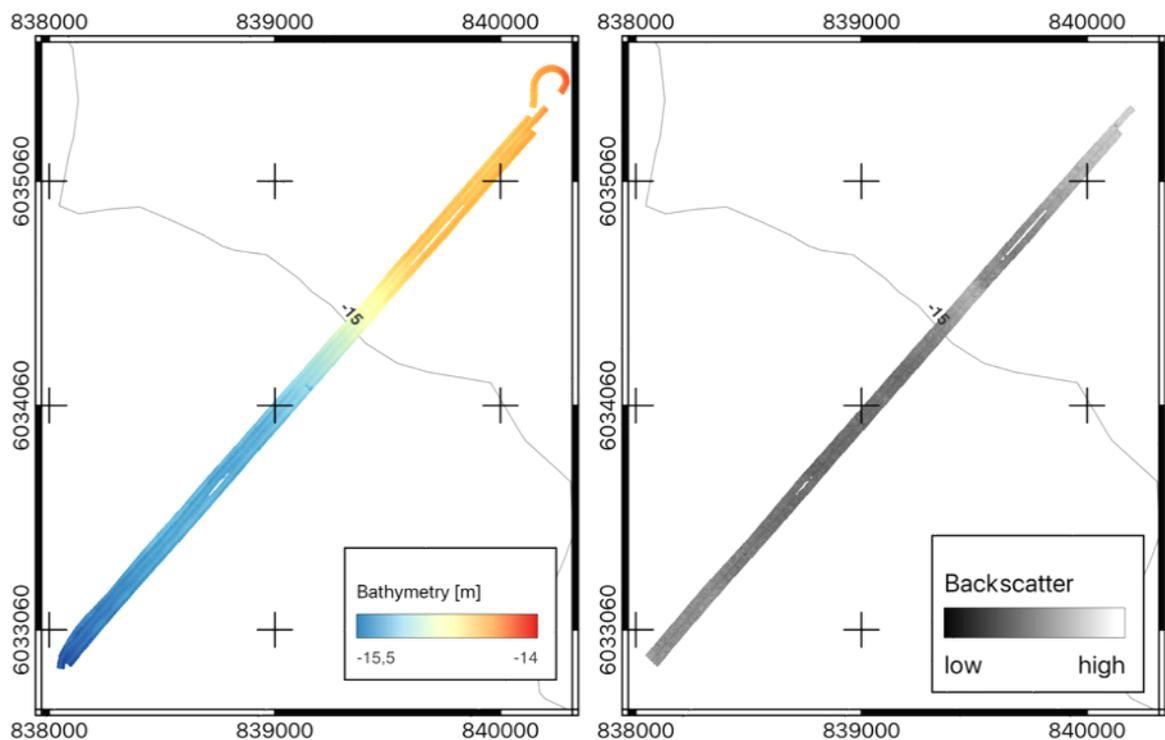
**Fig. 5.1.6** Bathymetric map (left) and backscatter map (right) of the ECOMAP area at Oder Bank area. No features are visible at the flat and smooth seafloor surface.
