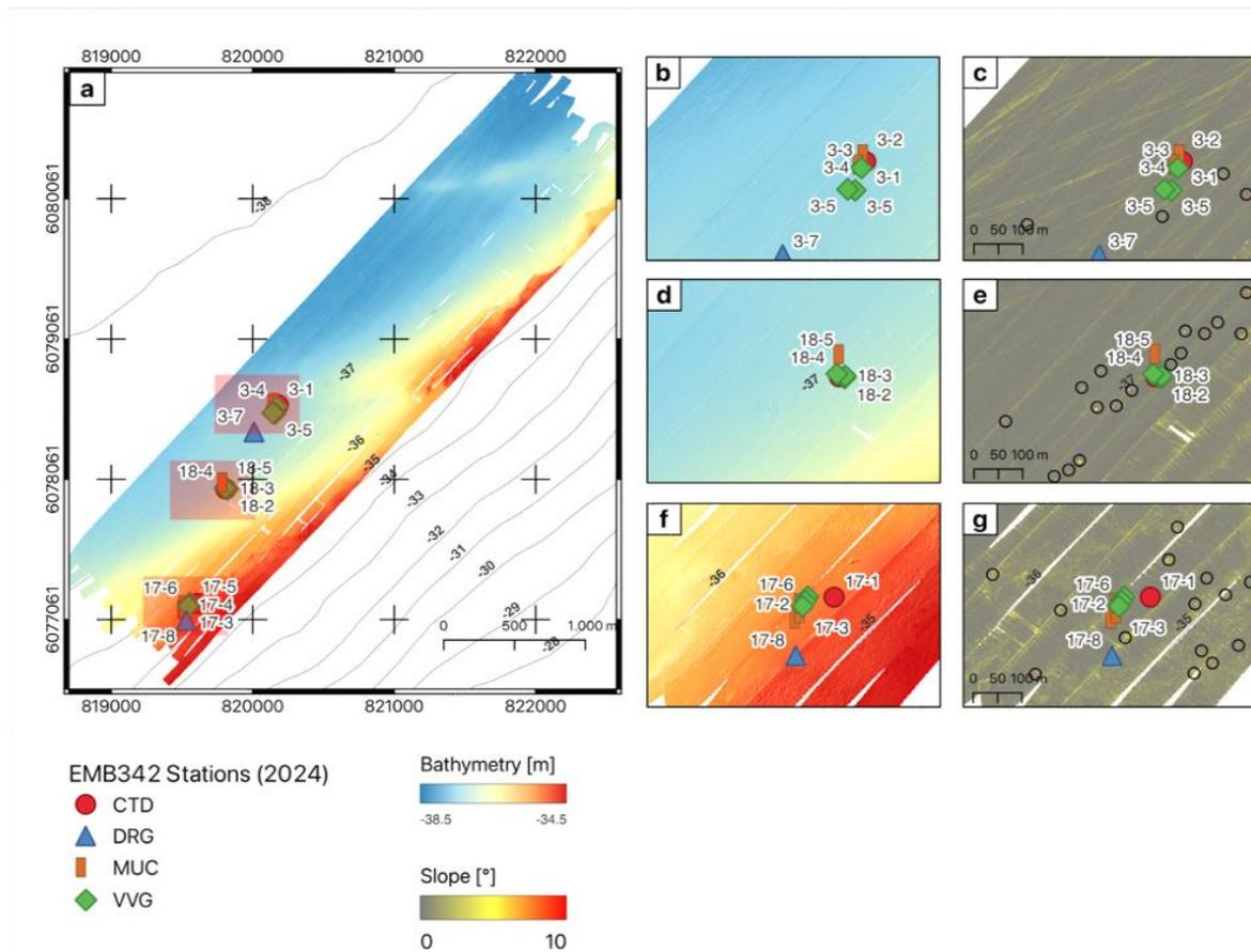
**Fig. 5.1.1** (a) Bathymetric map of Rönne Bank MPA area. The impact of trawl tracks on the seafloor surface is clearly visible in the bathymetry with hillshading (b, d, f) and slope data (c, e, g) at the respective stations. Circles mark some of the isolated stones of meter-scale diameter (b, d, f).
