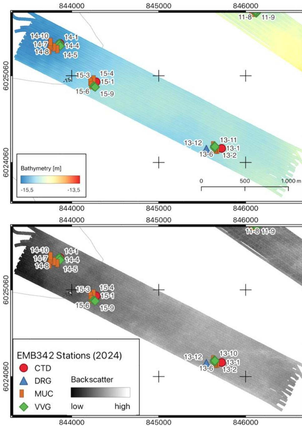
**Fig. 5.1.5** Bathymetric (upper) and backscatter (lower) map with hillshade of the REF area at Oder Bank area. No trawl marks are visible in the data.
