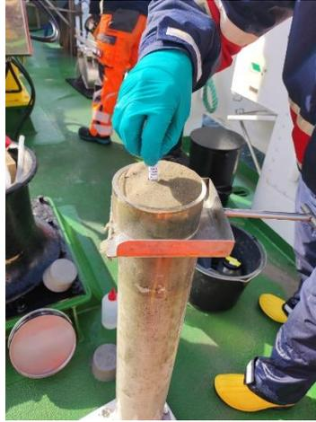
**Fig. 5.5.2** Taking eDNA samples of the sediments.
