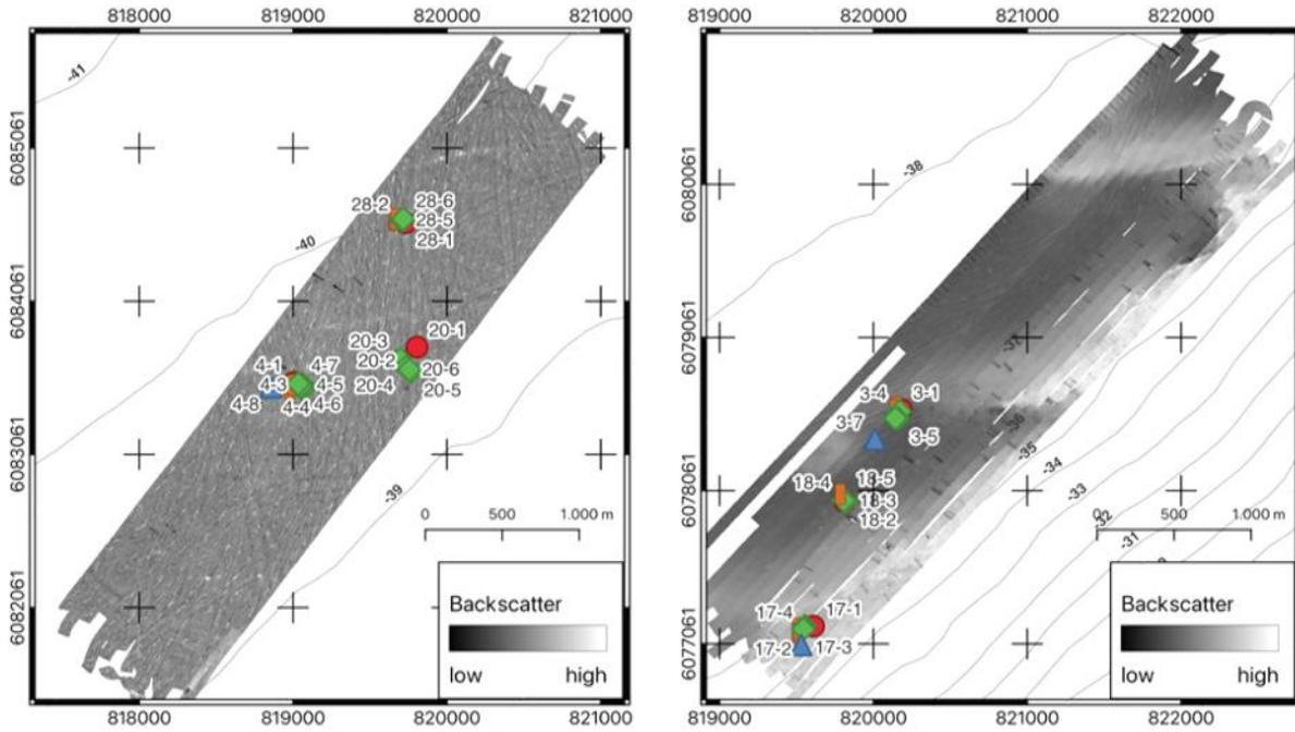
**Fig. 5.1.3** Backscatter maps of the REF area (left) and MPA (right) at Rönne Bank area with trawl marks present as described in the data before. Please note: this is a preliminary data processing.
