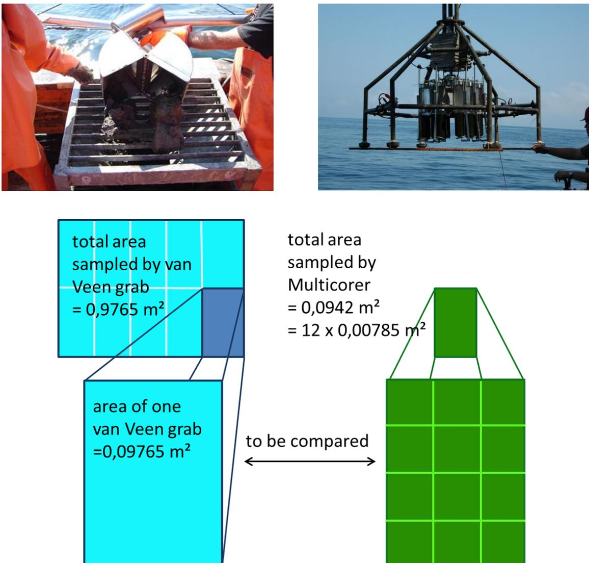
**Fig. 6.** Surface-sediment sampler used in this study a) van Veen grab sampler (pictured by IfAO) and b) Multicorer (pictured by Geomar). The planned and realized sampling design, of this investigation, with the areas sampled by van Veen grab and Multicorer.
