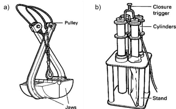
**Fig. 3. Surface-sediment sampler: a) van Veen grab sampler and b) Multicorer by Downing (1984).**
