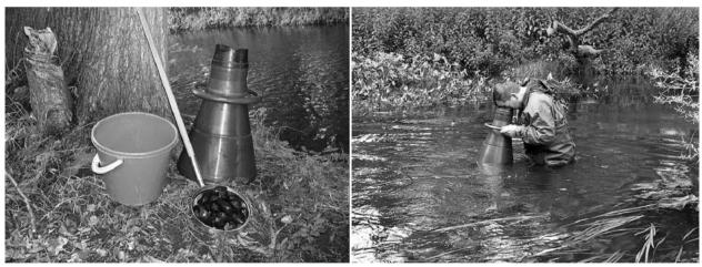
**Fig. 2**. The equipment for the monitoring of unionid mussels in running waters. On the left hand side a bucket for storage the mussels, a hand held screen for scraping gravel and sieving sandy substrates and a bathiscope for watching the mussel sipho openings at the sediment surface (see right).
