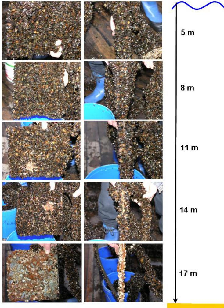
**Fig. 12.** Epibenthos on settling substrates in different water depths after 177 days of exposure in January 2005. The front and side views of the steel tiles show the increased density of organisms at water levels near the surface
