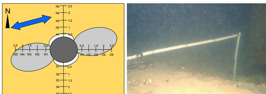
**Fig. 13.** Direction and spatial extent of sediment erosion (white area) and deposition (grey area) around the test cylinder (dark grey). After 246 days, an erosion depth of more than 40 cm at the cylinder walls could be recorded. The spatial pattern and intensity of the erosion/redeposition process is closely related to main direction of current and speed of current
