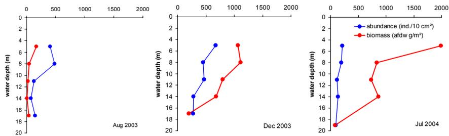
**Fig. 7.** Development of abundance (individuals per 10 cm<sup>2</sup>) and biomass (afdwt/m<sup>2</sup>) after 143 (left), 243 (middle) and 470 (right) days of exposure of steel plates in different water depths
