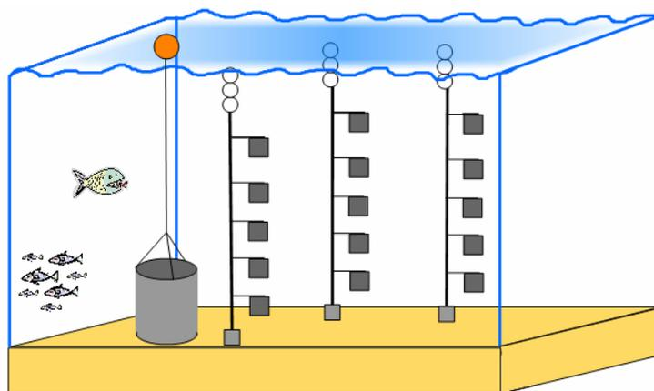
**Fig. 3.** Scheme of the experimental setup at the Darss-Sill station. On the left, note the permanently exposed steel cylinder, and on the right, the periodically exchanged steel settling substrates. Water depth is 20 m; the vertical distance between the artificial substrates is 3 m
