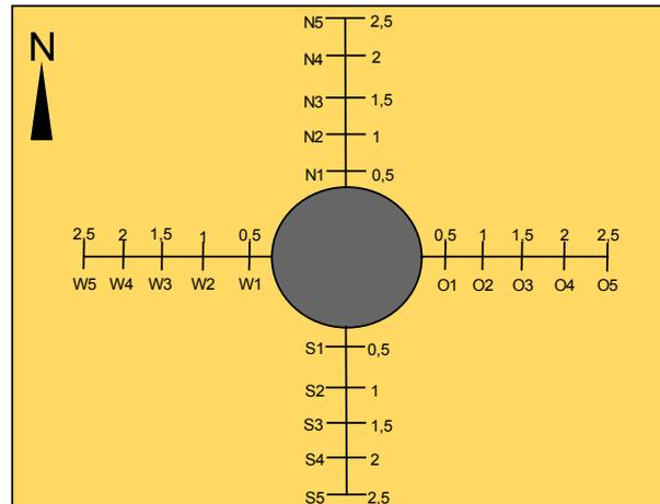
**Fig. 4.** The diver operated sediment sampling in May 2004 and March 2005 after 417 and 697 days of exposure followed the displayed scheme. The samples were taken at intervals of 0.5 m away from the central steel cylinder. Samples were labelled according to distance and direction
