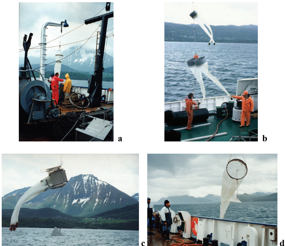
Figure 3.2.1: a , The WP-2 UNESCO Standard net being deployed aboard the R/V A. v. Humboldt; b , Twenty cm and 60 cm Bongo nets ready for deployment from the R/V Johan Hjort; c , The Multinet rigged for horizontal towing from aboard the R/V A. v. Humboldt; d , Deployment of a CalCOFI net from the R/V A. v. Humboldt. All photos stem from an ICES/GLOBEC Sea-going workshop for intercalibration of plankton samplers at Storfjorden, Norway, June 1993 (ICES, 2002).
