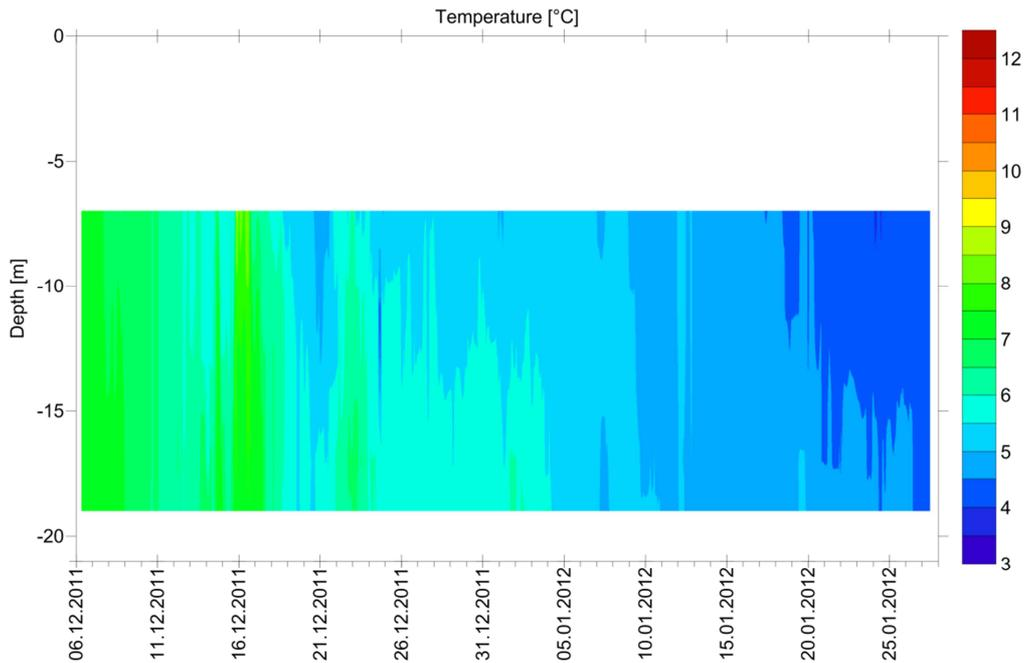
Figure 35: Temperature time series at the DSST mooring Darss Sill.
