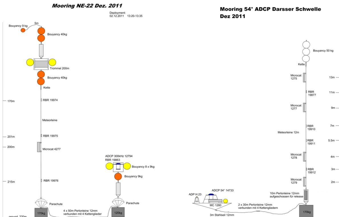
Figure 5: Sketch of the Gotland NE mooring (left) and the mooring deployed at the Darss Sill (right)
