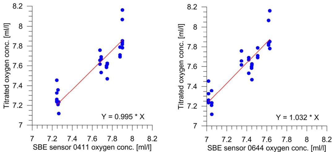
**Figure 4 Comparison between unvalidated CTD sensor oxygen concentration and Winkler titration of water samples (SN 411 left panel; SN 0644 right panel).**
