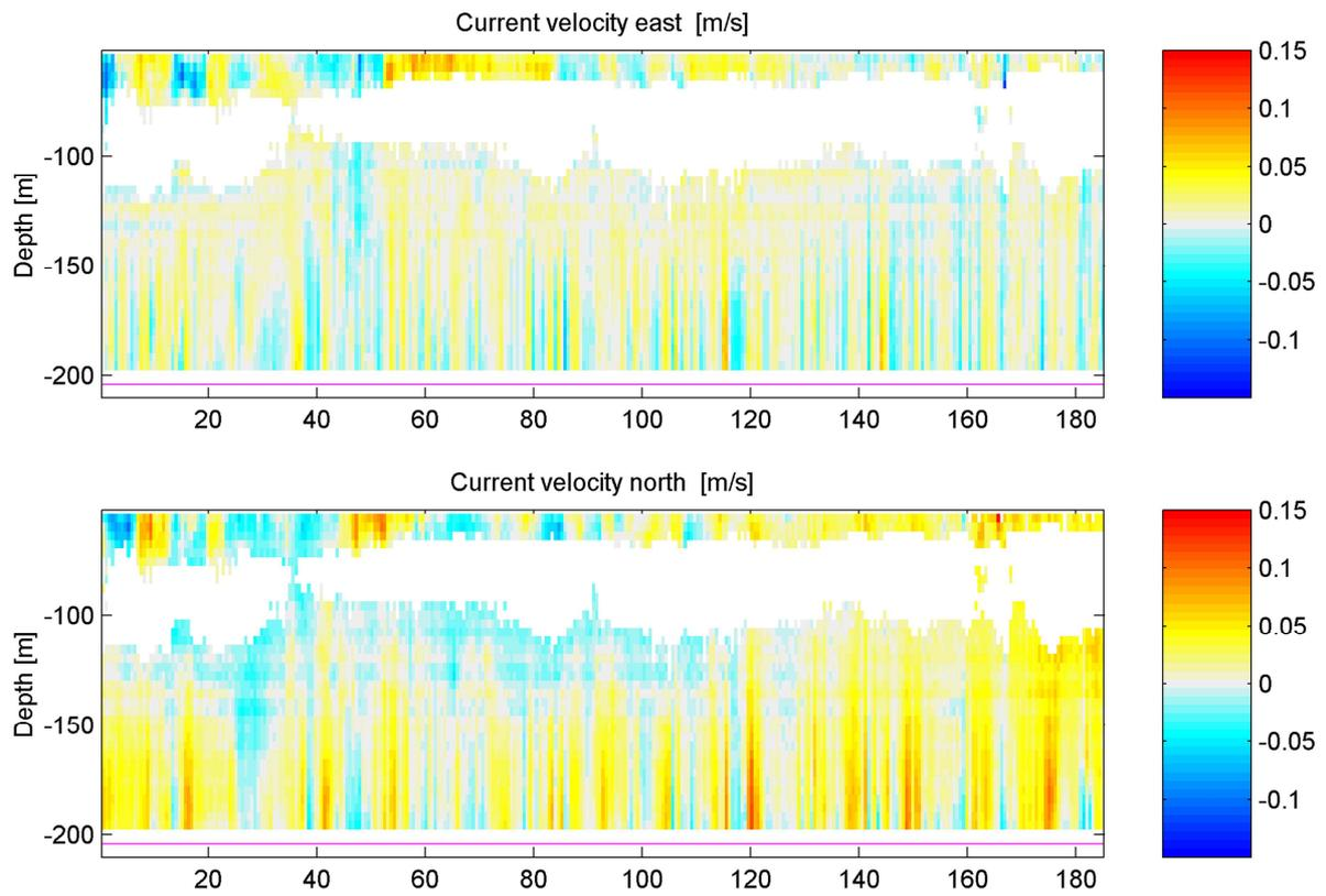
Figure 33: Time series of current measurements at the mooring position Gotland NE (01 April – 03 October 2011). The data are averaged over the inertial period (14 hours).
