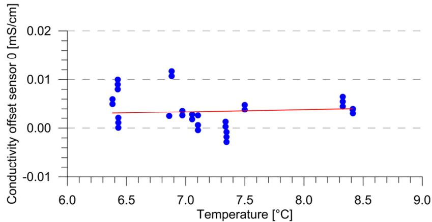
**Figure 3: Temperature dependence of conductivity offset for sensor 0**
