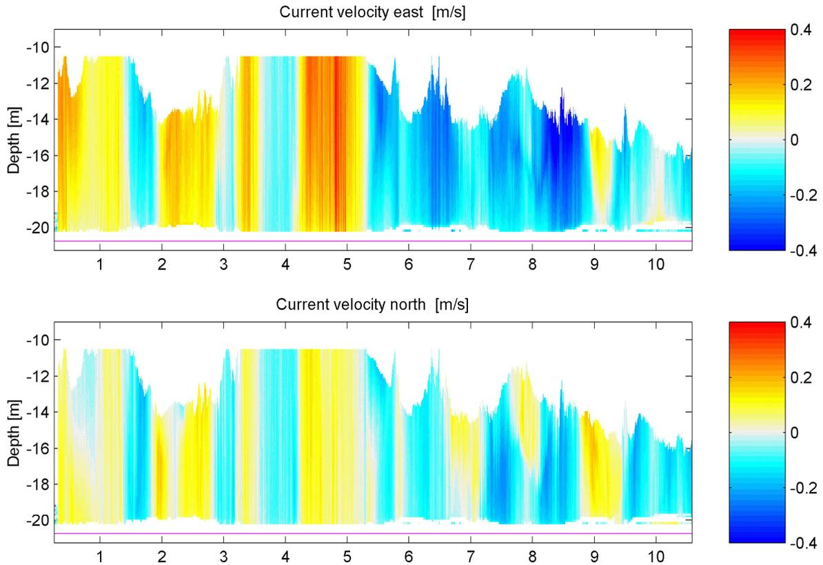
Figure 37: Current velocity at the Darss Sill. The x-axis is scaled in days after 6<sup>th</sup> Dec 2011 (1 = 7<sup>th</sup> Dec; 10 = 16<sup>th</sup> Dec)
