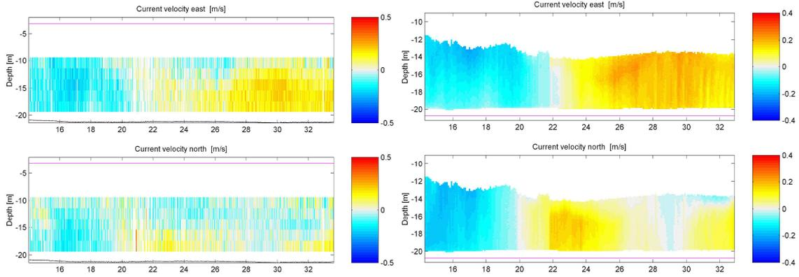
Figure 31: Current velocity at the Darss Sill during the time series measurements. Vessel mounted ADCP data (left) are biased to some amount by the ship in contrast to the undisturbed data from the 54° ADCP (right). The different color and depth scales have to be considered.
