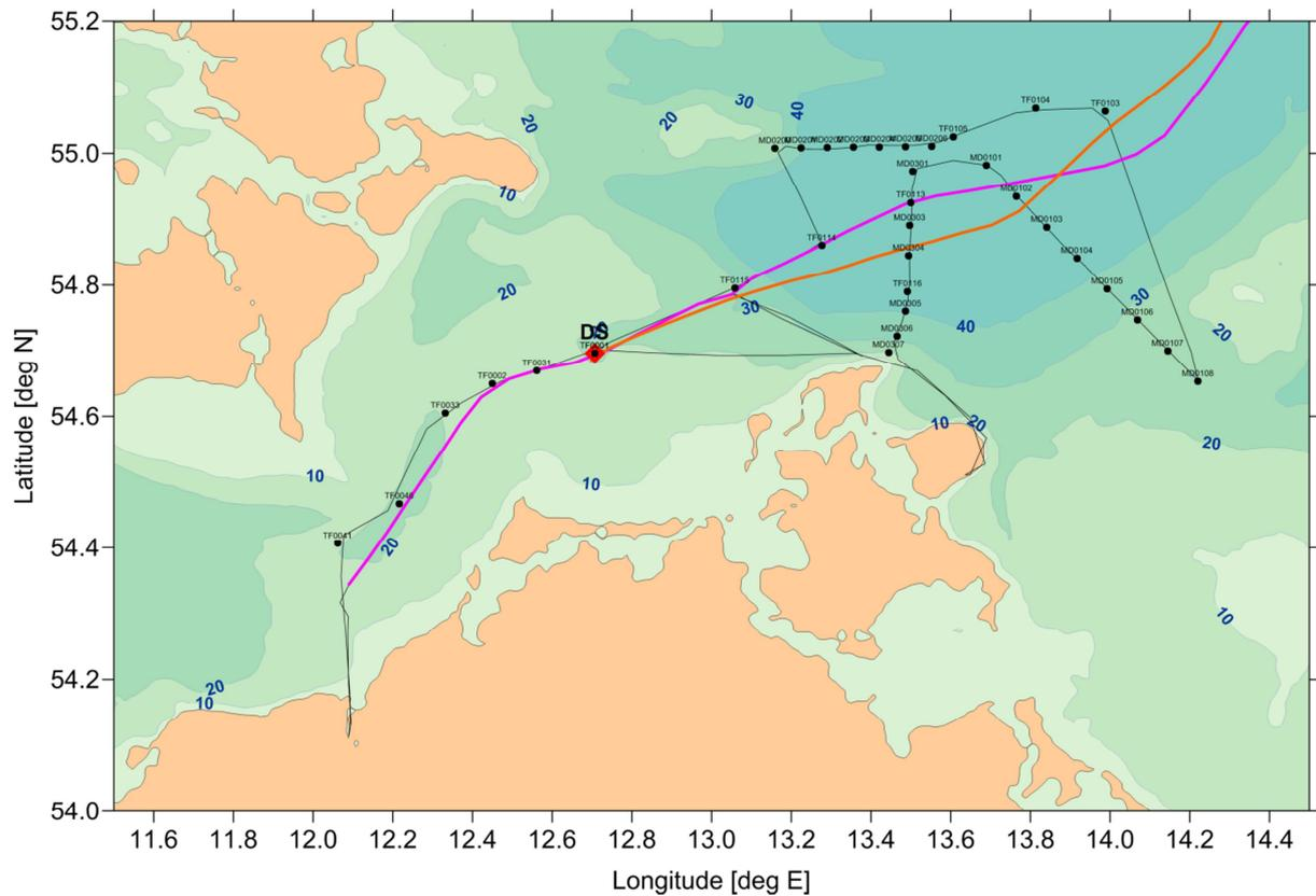
**Figure 2: Detailed map of stations and ship track (black line) in the Arkona basin. Black dots and labels indicate CTD stations, the magenta and orange lines depict the ScanFish transects, red diamond mark the mooring at the Darss Sill.**
