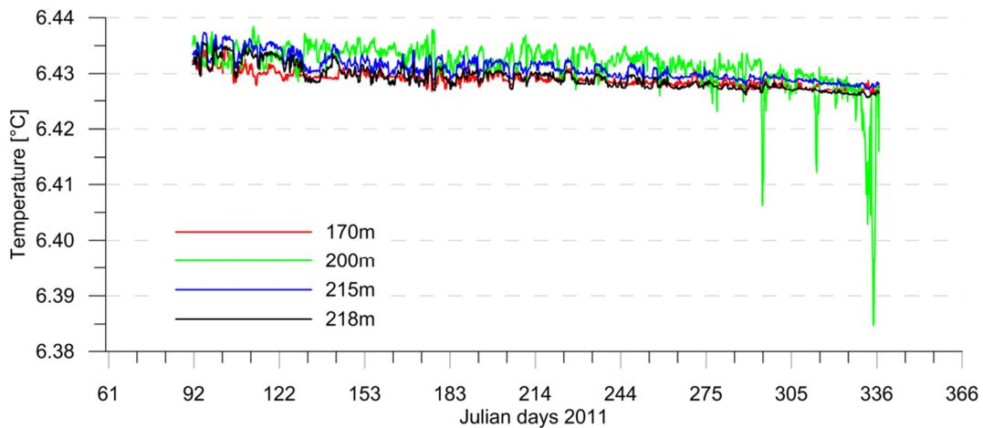
Figure 32: Temperature at different depth at the mooring position Gotland NE.
