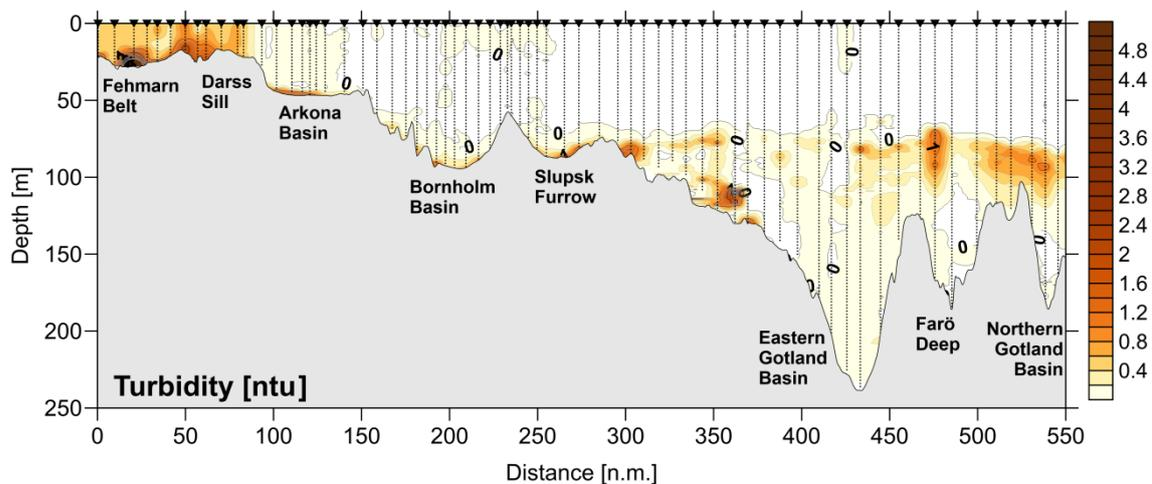
**Fig. 5.18** Distribution of turbidity along the talweg of the Baltic Sea from the Kiel bight to the northern Gotland Basin. The figure is based on the preliminary CTD data gathered from 15.03. - 23.03.2023.
