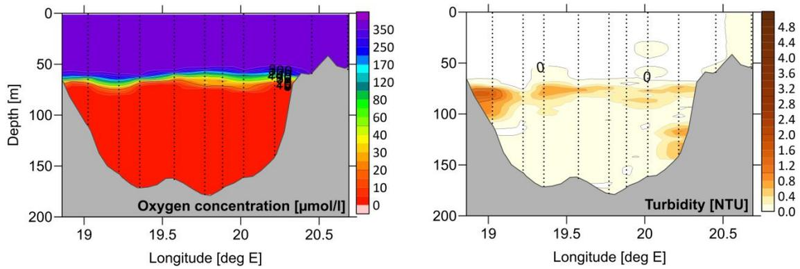
**Fig. 5.22** Dissolved oxygen and turbidity distribution along the zonal transect at the southern rim of the Eastern Gotland Basin (based on preliminary CTD data, 20./21.03.2023).
