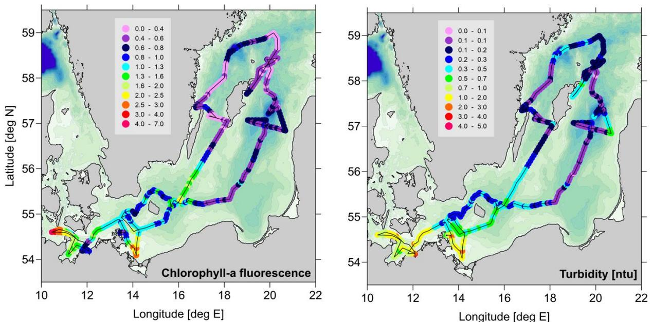
**Fig. 5.10** Surface chlorophyll-a fluorescence distribution (left) and distribution of surface turbidity (right) along the cruise track of EMB314 in the Baltic (30 min averaged values).
