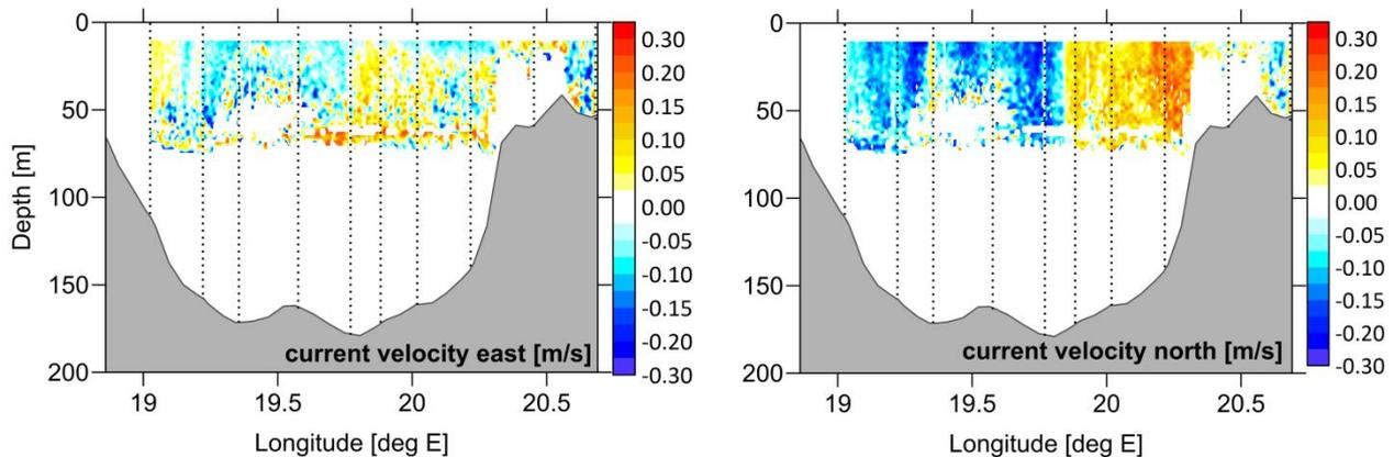
**Fig. 5.23** Current velocity distribution along the zonal transect at the southern rim of the Eastern Gotland Basin (based on preliminary VMADCP data, 20./21.03.2023).
