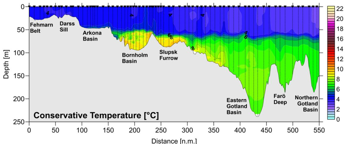
**Fig. 5.14** Distribution of conservative temperature along the talweg of the Baltic Sea from the Kiel bight to the northern Gotland Basin. The figure is based on the preliminary CTD data gathered from 15.03. - 23.03.2023.
