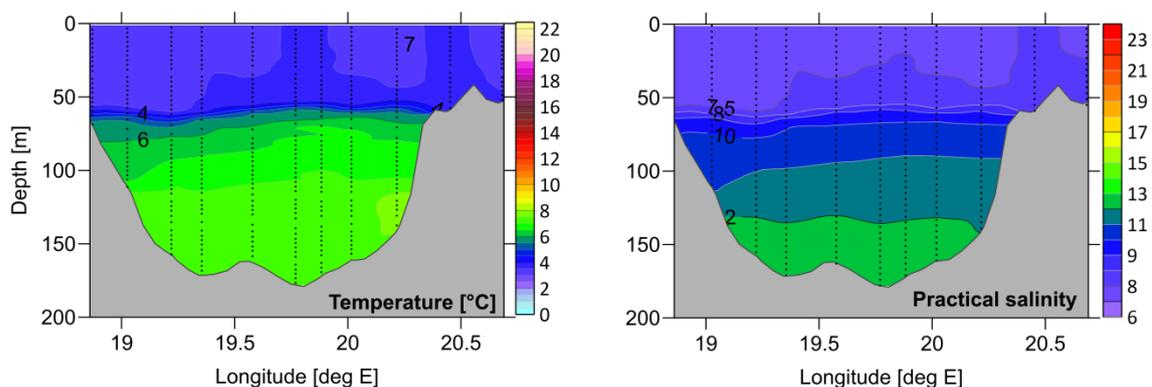
**Fig. 5.21** Temperature and salinity distribution along the zonal transect at the southern rim of the Eastern Gotland Basin (based on preliminary CTD data, 20./21.03.2023).
