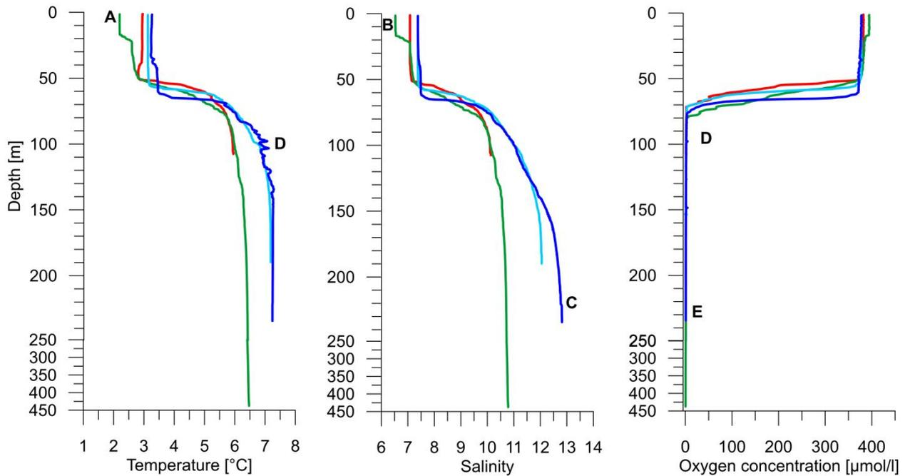
**Fig. 5.19** Vertical profiles of temperature, salinity and oxygen concentration (CTD data) at the main stations in the central Baltic. Gotland Deep TF0271 (blue), Farö Deep TF0286 (cyan), Landsort Deep TF0284 (green), and Karlsö Deep TF0245 (red).
