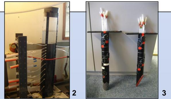
Fig. 2 and 3: Pore water sampling via rhizons (2) and groundwater lances (3).
