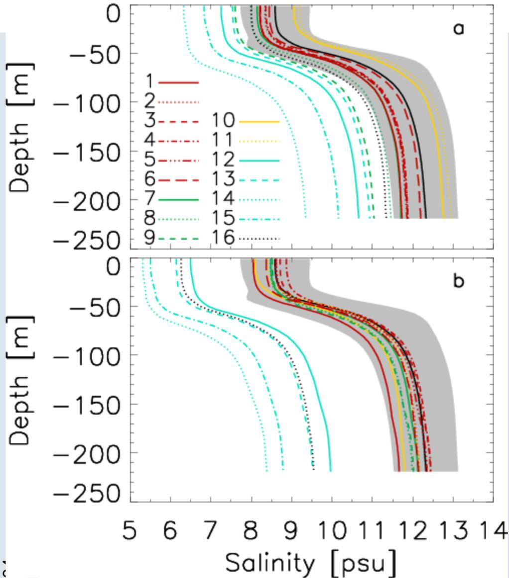
Median profiles of salinity at monitoring station BY15 for present climate 1961-1990 (black solid line, shaded areas indicate the  $\pm 2$  standard deviation band calculated from two-daily values for 1903-1998) and in projections for 2071-2100 (colored lines). In (a) only effects from wind changes are considered whereas in (b) projections based upon wind and freshwater inflow changes are shown. Numbers in the legend correspond to different scenario runs (Meier et al. 2006).
