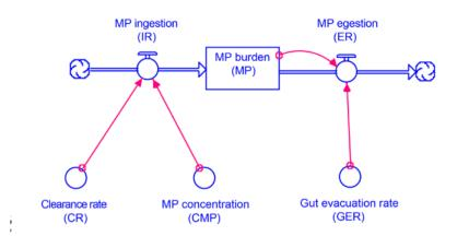
Figure 1. Schematic representation of the model by Ogonowski et al. (2019) developed to predict microplastic body burden (MP burden) in the Baltic herring using food intake by fish estimated from clearance rate (CR), ambient microplastic concentration in the water column (CMP) and gut evacuation rate of the fish (GER).
