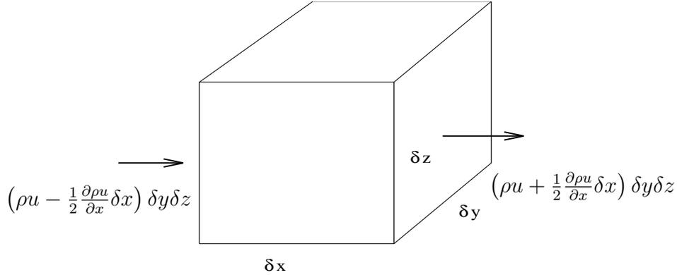
Figure 2.2. Budget of mass for a flow through a volume element
