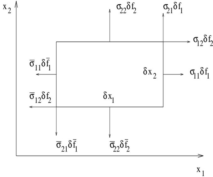
Figure 2.3. Forces acting on the surface of a parallelepipeds.
