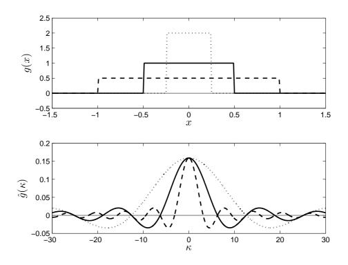
Figure 1: Function g(x) and Fourier transform  $\hat{g}(\kappa)$  of a symmetric box window with different  $H = 1/\Delta$ .
