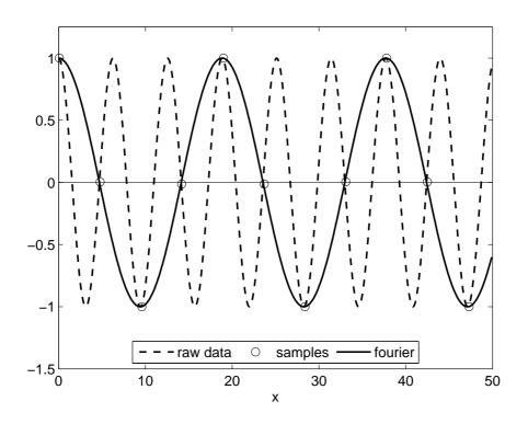
Figure 4: Example of aliasing of a raw signal (dashed line) by undersampling (circles) creating a false frequency (solid line).
