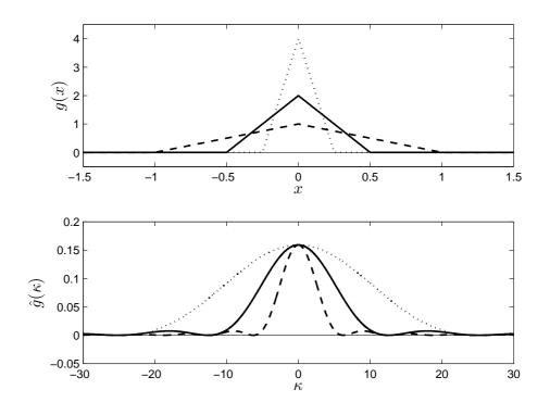
Figure 2: Function g(x) and Fourier transform  $\hat{g}(\kappa)$  of a symmetric Bartlett window with different  $H = 2/\Delta$ .
