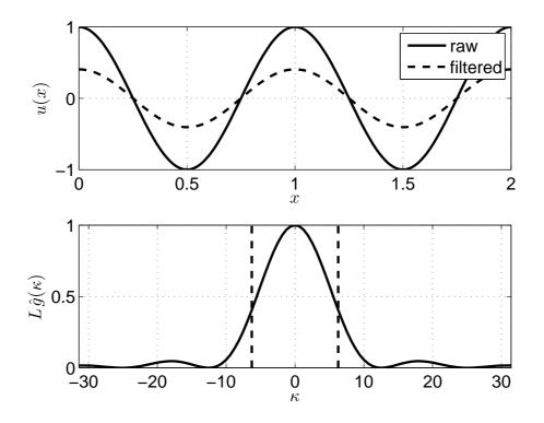
Figure 3: Raw and filtered signals (upper panel), and Fourier transform  $\hat{g}(\kappa_m)$  of the Bartlett filtering window (lower panel). The vertical dashed lines in the lower panel indicate the wave number  $\kappa_m$  of the signal.
