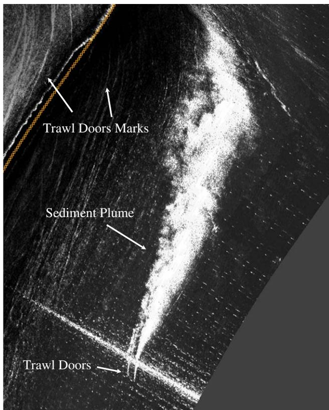
Fig. 8. An active shrimp trawling rig in the Galveston ship channel imaged by side scan sonar. Note that the trawl doors produce the majority of the suspended sediment plume. The image also shows how the plume rapidly expands after the passage of the trawl rig. Most of the light lineations in the image are older trawl door marks.
