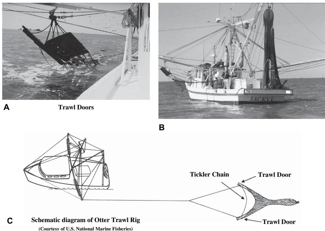
Fig. 2. Shrimp trawling rig, (A) with trawl doors of a bait trawling rig; (B) a suspended trawl net, the circular object at the top of the net is the turtle exclusionary device (TED). (C) The schematics of a typical trawling rig underway, showing all of the tickler chain and trawl doors.
