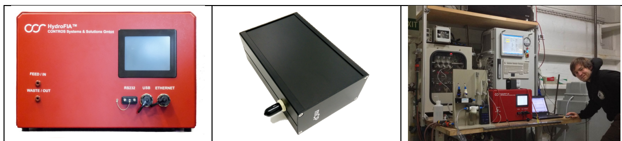
Fig. 1: Left – first prototype of the spectrophotometric pH-measurement system; Middle – cartridge containing the dye solution; Right – picture of the field test with the first prototype developed within PINBAL in front, IOW's permanent pCO 2 -measurement system in the back, and PINBAL PhD-student Jens Müller, operating the system, on the right.
