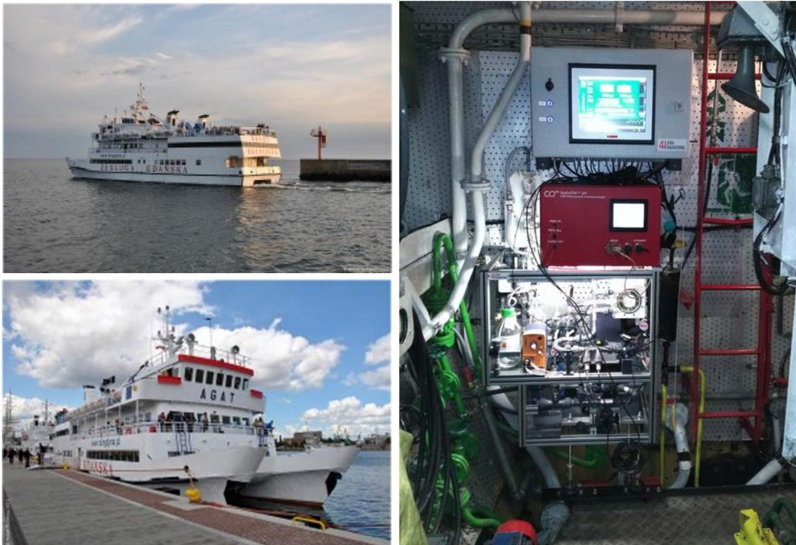
*Figure 13: upper and lower left - m/s AGAT (source: [www.naszbaltyk.com](http://www.naszbaltyk.com)), right - ferrybox installed in the engine room of m/s AGAT.*
