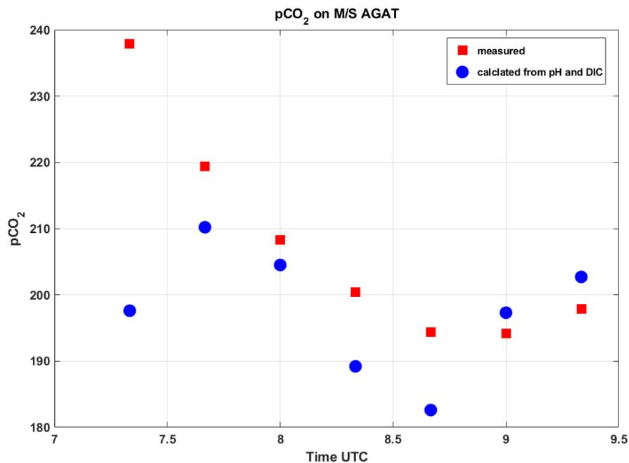
**Figure 14:** Results of the crosscheck experiment performed on m/s AGAT in May 2018. Comparison of the  $p\text{CO}_2$  measured (red dots) and calculated from DIC and pH (blue dots).
