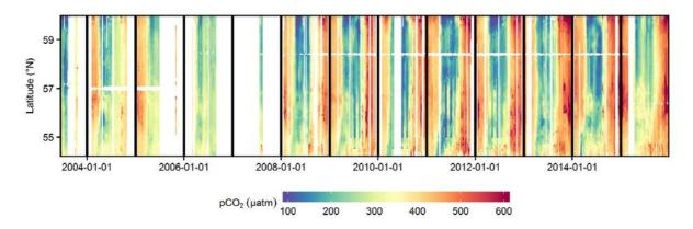
Figure 5: Compiled pCO₂ data between 2003 and 2016 between Lübeck (lowest part of panel) and Helsinki (uppermost part of panel) gathered on VOS Finnmaid. For cruise track information, refer to Figure 4 (VOS Finnmaid). Plot from Schneider and Müller, 2018.
