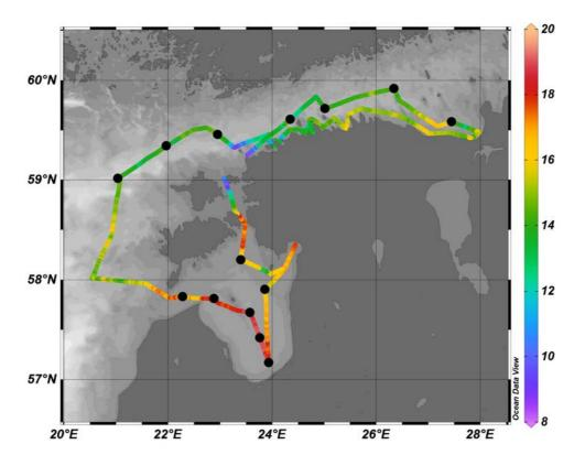
**Figure 10:** RV SALME track during the monitoring / BONUS INTEGRAL cruise on May 28 – June 2, 2018. Colour scale shows surface water temperature (in degC, water intake at 2 m depth) recorded by the flow-through system. Black dots indicate monitoring stations where additional water sampling for BONUS INTEGRAL analyses is conducted.
