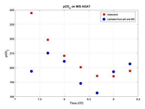
**Figure 14:** Results of the crosscheck experiment performed on m/s AGAT in May 2018. Comparison of the pCO<sub>2</sub> measured (red dots) and calculated from DIC and pH (blue dots).
