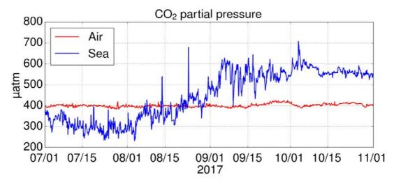
**Figure 8:** Atmospheric and sea water carbon dioxide partial pressures at Utö during the period of 1 July – 1 November 2017 (Honkanen et al., 2018). During the summer period, the sea water pCO<sub>2</sub>-concentration is lower than the atmospheric concentration due to the biological carbon sink. Atmospheric CO<sub>2</sub>-observations at Utö are part of ICOS.
