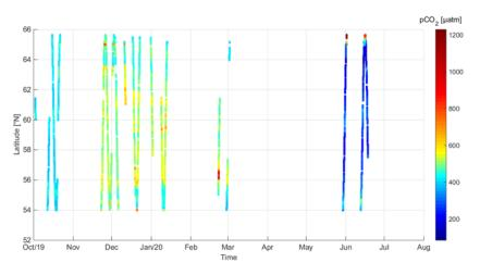
*Figure3:* Data of seawater  $pCO_2$  from October 2019 until July 2020 recorded by the SOOP Tavastland. Data gaps are mainly due to pump problems. The huge gap in spring 2020 was caused by the Covid-19 pandemic as maintenance on board was not allowed. Data given against latitude. For cruise track information, see Fig. 1.
