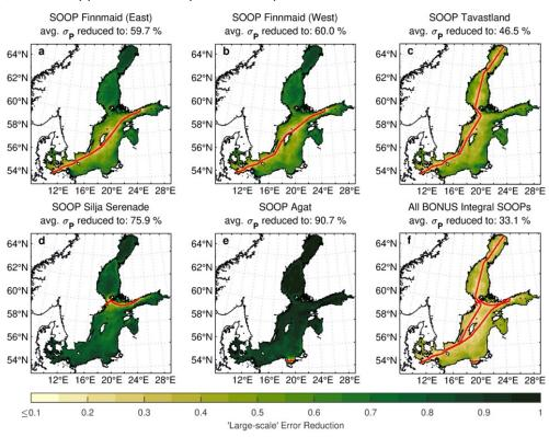
**Figure 4:** Reduction in large-scale error by SOOP line surface  $pCO_2$  sampling for (a) Finnmaid on Eastern route, (b) Finnmaid on Western route, (c) Tavastland, (d) Silja Serenade, (e) Agat, and (f) all SOOP lines of BONUS INTEGRAL combined (with an assumed common 5 µatm observation error).
