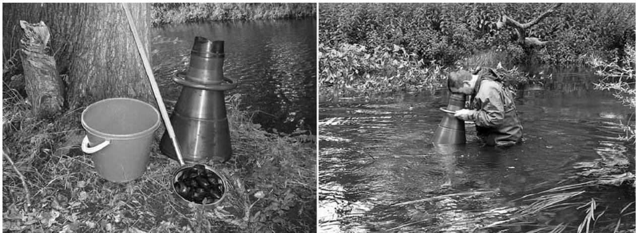
**Fig. 2.** The equipment for the monitoring of unionid mussels in running waters. On the left hand side a bucket for storage the mussels, a hand held screen for scraping gravel and sieving sandy substrates and a bathyscope for watching the mussel siphon openings at the sediment surface (see right).
