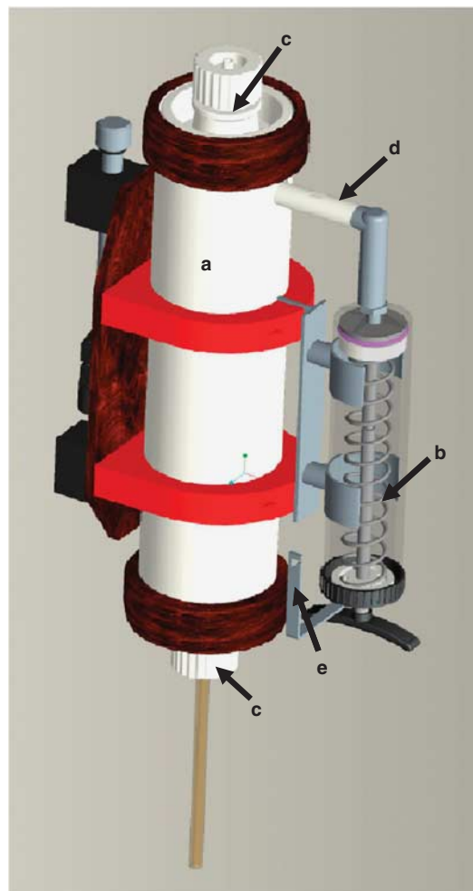
Figure 2 Design of the AFIS. (a) Teflon water bottle (2.7 l volume); (b) syringe (hand syringe GENIUS 450 ml) with maximal volume of 300 ml; (c) bottle lids connected with closing devices on the CTD-bottle rosette; (d) adapter between syringe and bottle, coupled with a dispenser tube; (e) escapement for the syringe plunger, directly connected with the closing devices for the bottle lids. The operating mode is based on the following principles: (1) the syringe plunger is pushed by a spring; (2) the release of the spring is coupled with the closing devices for the bottle lids; (3) the solution passes through the dispenser tube into the bottle; (4) the dispenser tube extends from the top to the bottom of the bottle; (5) the solution is equally distributed through perforations of increasing diameters made in the dispenser tube.
