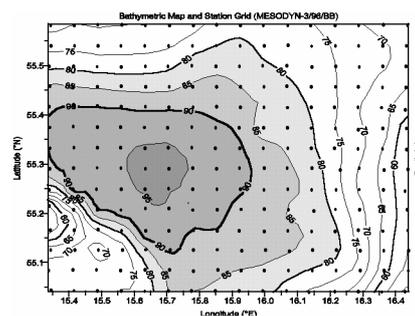
Fig.2 Bathymetric map (m) resulting from echosoundings at 224 hydrographic stations (dots) with the spacing of 2.5 n.m. above the Bornholm Basin during 03 -13 June, 1996.
