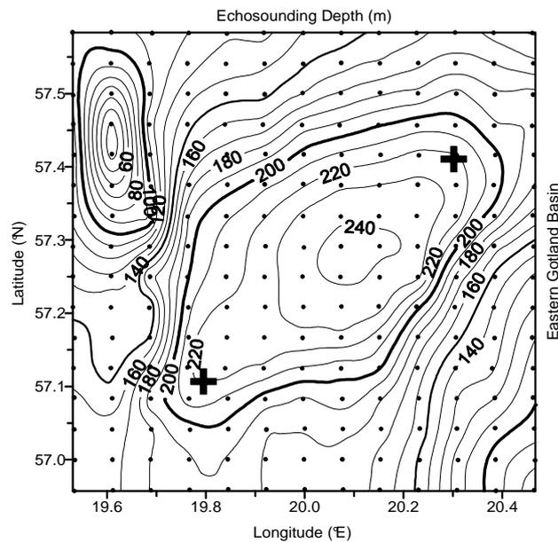
Fig.2 Bathymetric map of the MESODYN-7 area with positions (crosses) of two subsurface moorings each with three current meters (RCM-7) at 215m, 200m, and 170m above the sea bed at 220m; the top of the mooring locates at 130m depth; recovering is planned in May 1998; dots indicate hydrographic stations.
