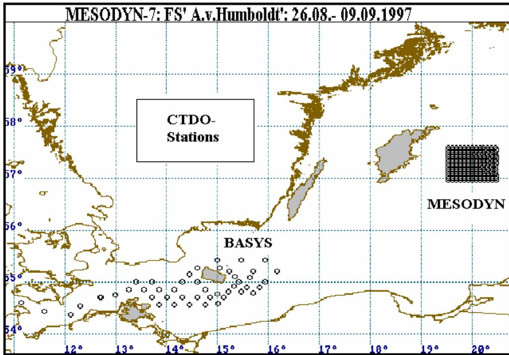
Fig.1 Hydrographic station map for the MEDODYN-7 field campaign carried out with R/V 'A.v.Humboldt'. The station spacing was 2.5 n.m. above the eastern Gotland Basin (EGB) but somewhat larger in the Bornhom & Arkona Basin. These irregularly arranged stations are part of a tracer-experiment performed for BASYS by the BSH-Hamburg (released by R/V 'Gauss', cruise -291, 1997) in co-operation with the Institute of Marine Research of the University of Hamburg.
