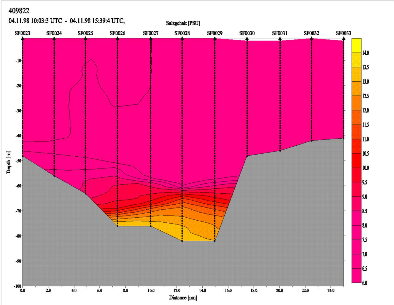
Fig. 11 Salinity Distribution on a Meridional Section along 17°35'E in the 2.Phase
