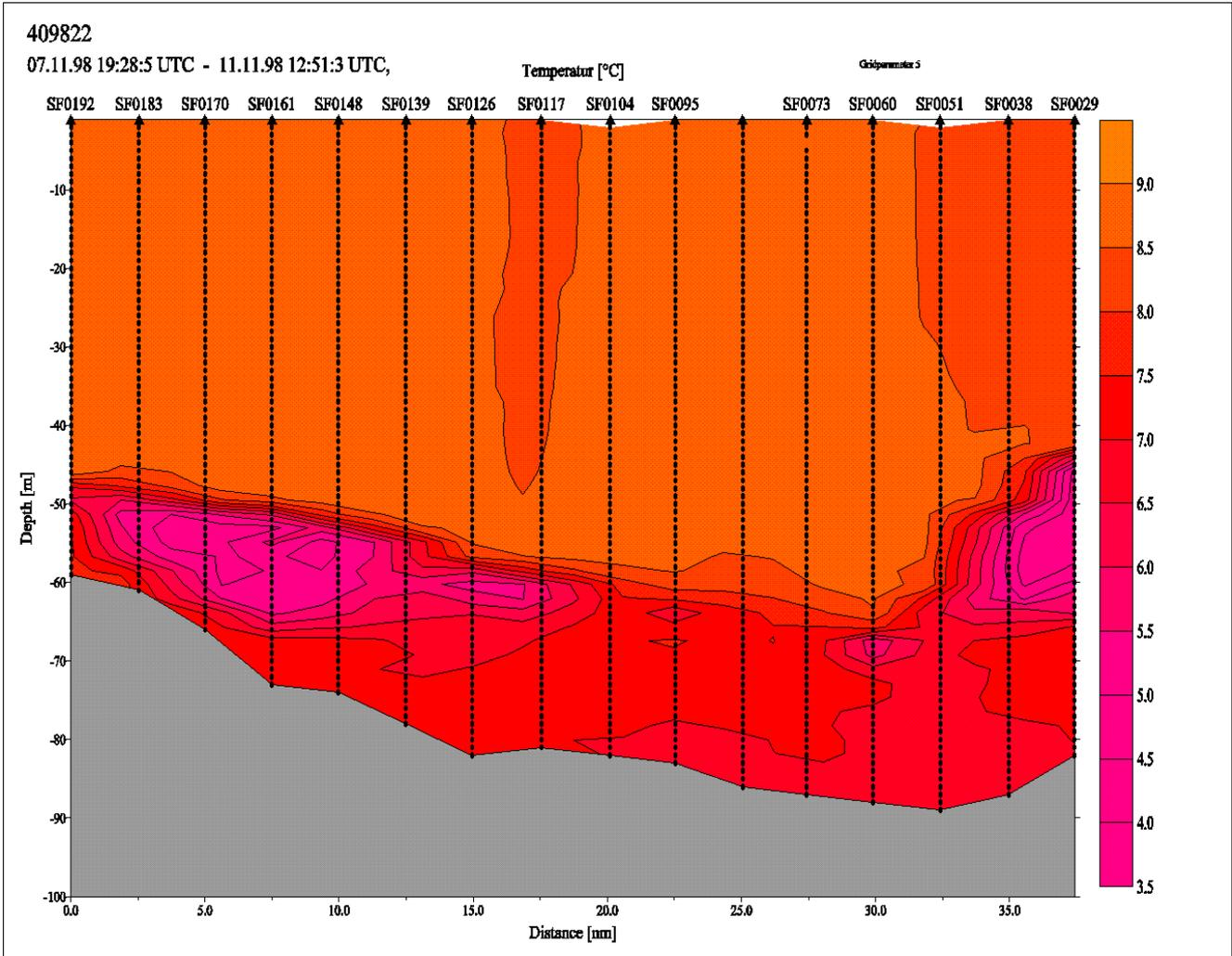
Fig. 8 Temperature Distribution on a Meridional Section along 17°35'E in the 1.Phase
