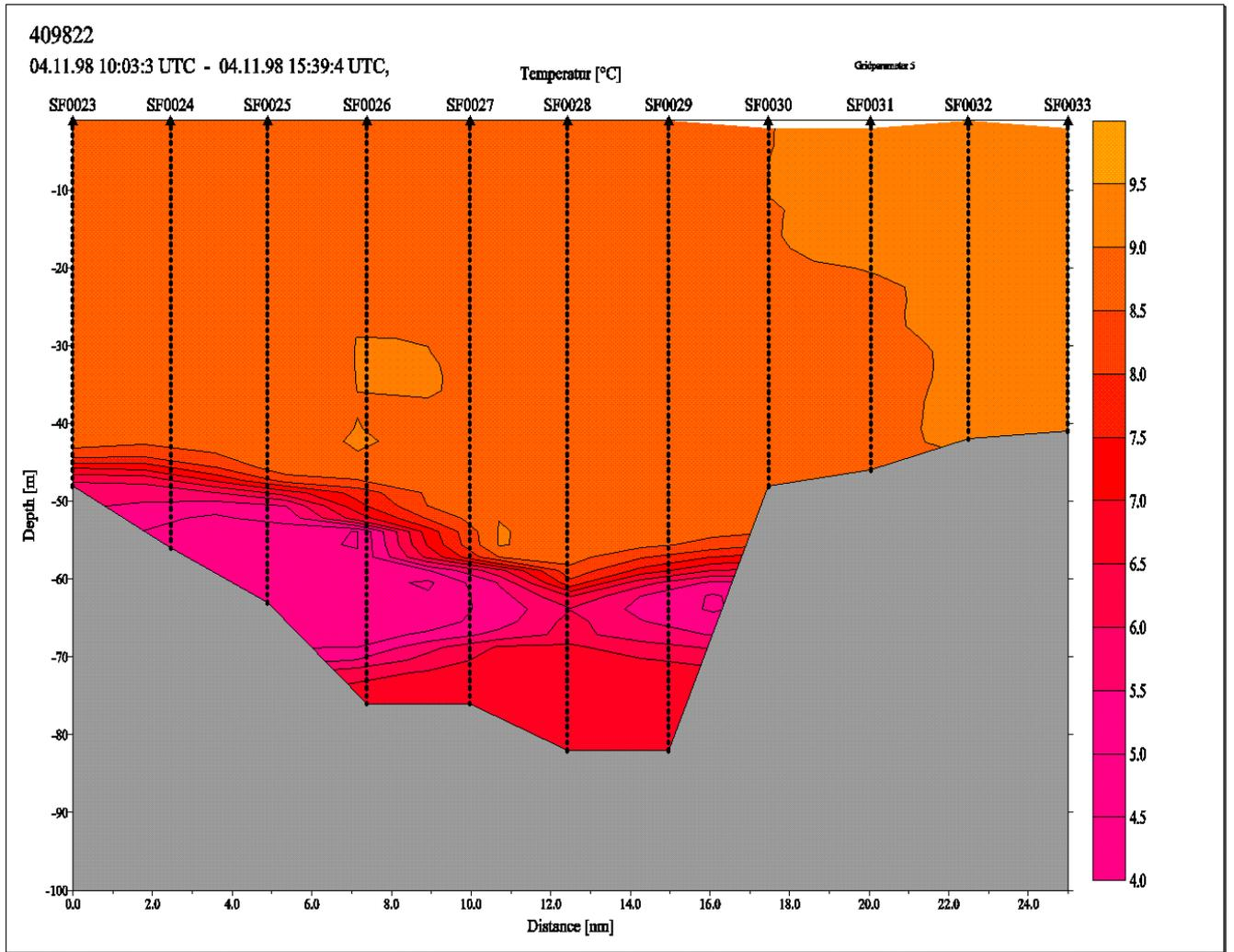
Fig. 9 Temperature Distribution on a Meridional Section along 17°35'E in the 2.Phase
